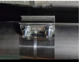
4. The pipeline installation should be moderately tight, and the new exhaust system should be adjusted to meet the clearance and appearance requirements. Tighten all connections and fixtures evenly, starting from the front flange connection and then proceeding with the subsequent connections.
