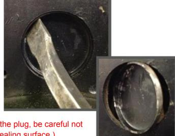
(Note: Do not tap the center of the plug, be careful not to scratch the plug, as it is a sealing surface.)
